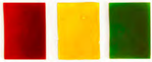
Caramelized sugar coated with beeswax. Samples were heated to various high temperatures during preparation.
